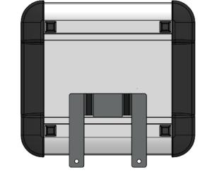
Hang the other bracket from the back of the controller in the location shown here.
