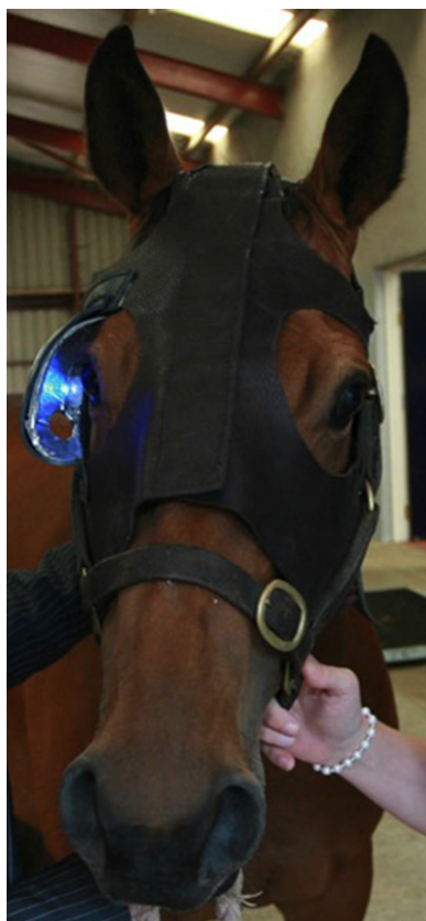
Fig 1: A horse wearing the light mask that provided 50 lux blue light to the right eye. The light mask consists of a leather headpiece with a semi-rigid rubber cup containing a single blue-light emitting diode fitted on the inside of the rubber eye cup. The inner surface of the cup is covered with reflective aluminium foil to reflect light diffusely onto the eye. A Velcro fastening down the centre of the face permits adjustability.
